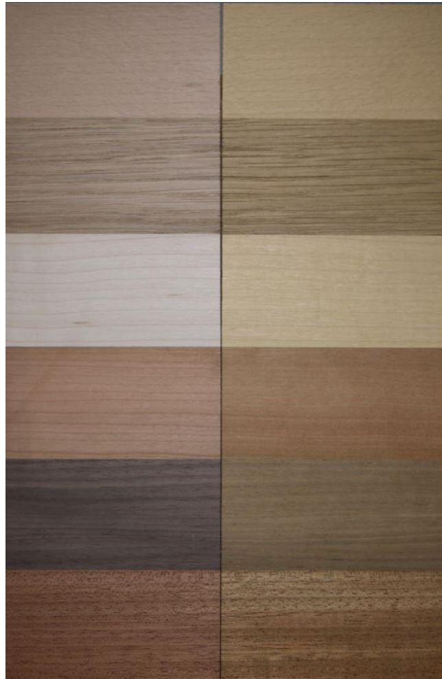
Figure: Lightened bare woods. From top to bottom: beech, oak, maple, cherry tree, walnut and mahogany. The right half have been lightened (Atlas sun test).
