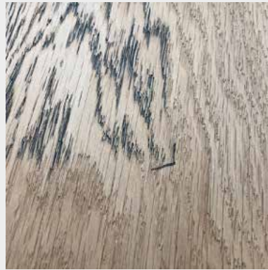
Figure 1: Depiction of the discolouration of open-pored wood under the influence of moisture (made visible using an iron solution).
