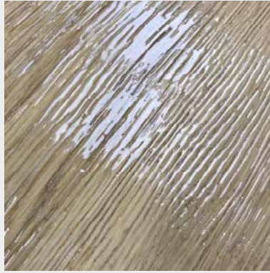
Figure 3: Open-pore wood after the first step in the POREGUARD procedure.
