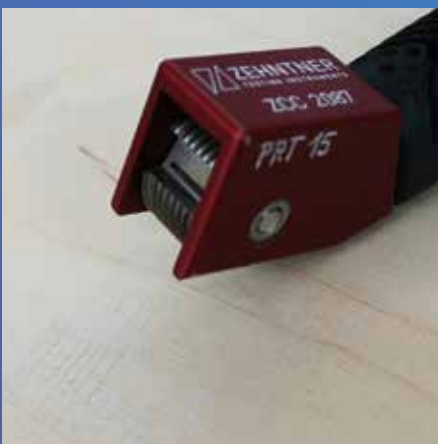
Cross cutting test (according to DIN EN ISO 2409): examination of the bond
