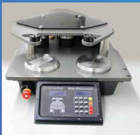
Micro-scratching according to EN 16094 applications: laminate, floor coverings, high-pressure laminate, high-gloss or polished surfaces
