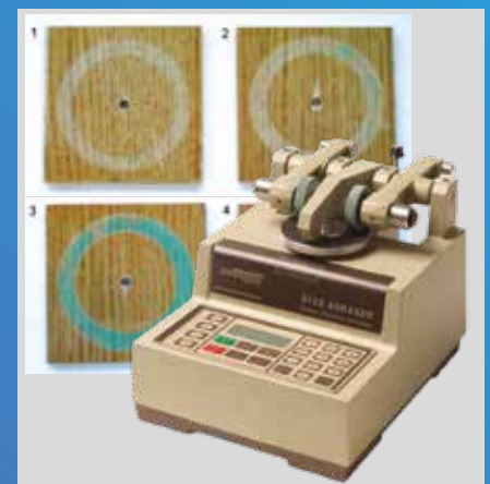
Taber test: determination of abrasion resistance according to various standards
