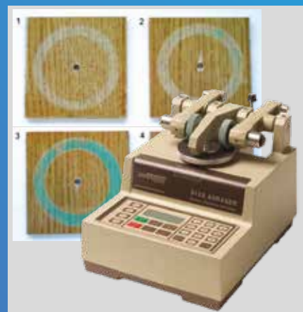
Taber test: determination of abrasion resistance according to various standards
